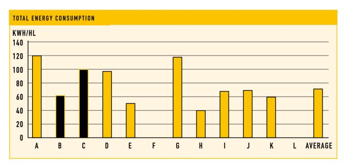
Total energy consumption for heat and electricity in kWh/hl from 10 of the 12 microbreweries in the survey for 2011. Black columns represent breweries without small pack filling lines.
